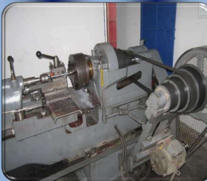
CENTRE LATHE MACHINE MAKE: ATUL [GUJARAT] CAPACITY: 5.5FEET
