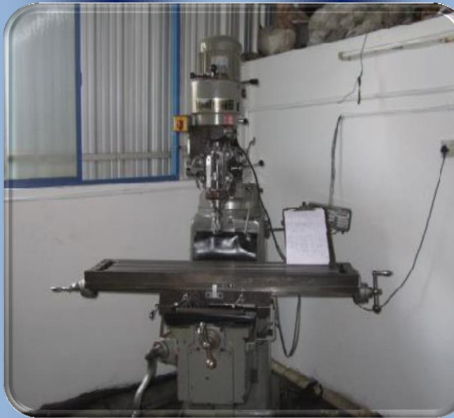
M1TR MILLING MACHINE MAKE: ARGO [TAIWA] CAPACITY: 3 KS with DRO
