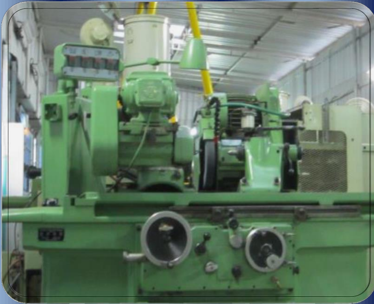
CYLINDRICAL GRINDING MACHINE MAKE: JONES-SHIPMAN [GERMANY] CAPACITY: 500mm length
