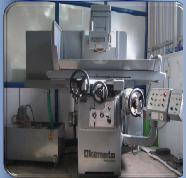
SURFACE GRINDING MAKE: OKAMOTO [JAPAN] CAPACITY: 250*550mm
